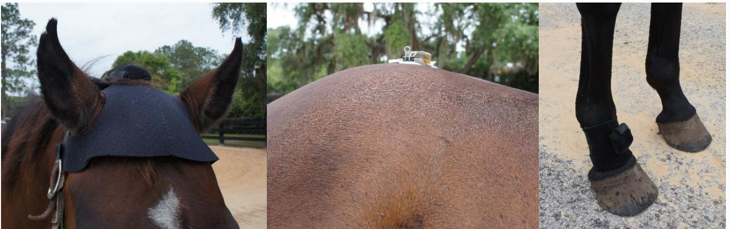
Small accelerometers are attached to a head bonnet, and a sticky pad on the pelvis. A gyroscope is attached with a wrap to the right front pastern.
